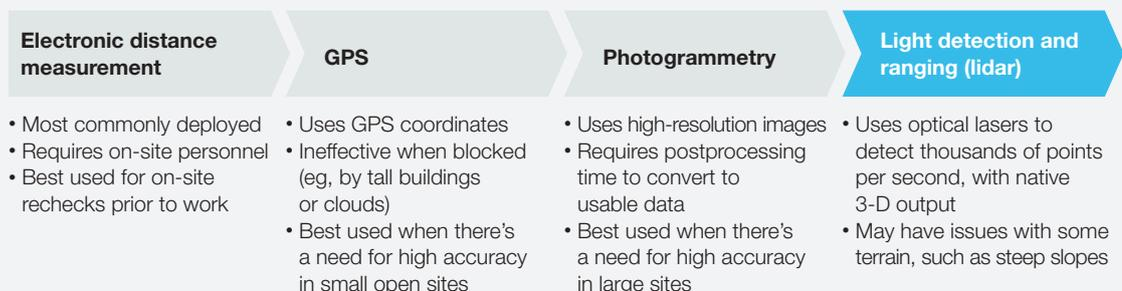
**While lidar has existed for some time, there has been a breakthrough in its use via drones/unmanned aerial vehicles (UAVs) and handheld platforms**
